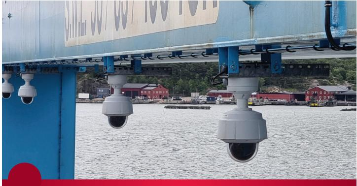
Visy utilizes durable PTZ cameras which are configured to cover multiple imaging areas. This ensures comprehensive support for all lifting cases and operation types.
