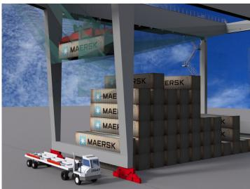
The OCR system and integrations cover and record the entire container handling process, while the box is lifted from the stack, train, or terminal tractor.
