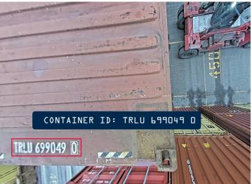
With Visy TopView, no containers are stacked or loaded to a wrong location. By confirming each container move with TopView, container handling procedures become more visible and accurate. This brings reliability to box moves if exception handling cases occur.
